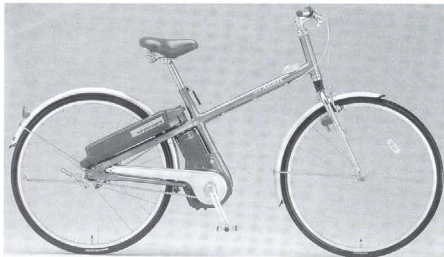
The state-of-the-art in 1997 is illustrated by the jointly developed Yamaha/Bridgestone "cross framed" bicycle with aluminium parts and 26-inch wheels with sprung front forks. This PAB weighs 26 kg, will travel 28 km on a single battery charge, has a power output of 235 watts and is recharged in 3.5 hours from mains electricity. Retail price in Japan with exclusive battery charger, A$1550.
