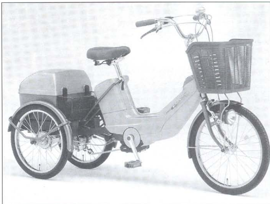
This Yamaha electric shopping tricycle has excellent stability and load carrying power. Battery charging takes 2.8 hours and will carry the rider 35 km on flat roads. Electronic indicators show battery levels and a dynamo light is fitted that stays bright at low speeds. It comes complete with a front wheel lock, comfortable sprung saddle and front basket. Retail price in Japan A$3550
