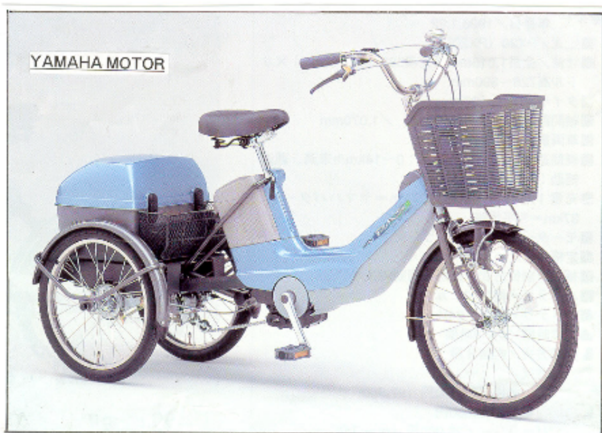
Figure 7 This Yamaha electric shopping tricycle has excellent stability and load carrying power. Battery charging takes 2.8 hours and it will carry the rider 35 km on flat roads. Electronic indicators show battery levels and a dynamo light is fitted that stays bright at low speeds. It comes complete with a built in front wheel lock, comfortable sprung saddle and front basket. This model weighing 36 kg is no longer available but the Bridgestone shopping tricycle that weighs 8 kg less is now available.
