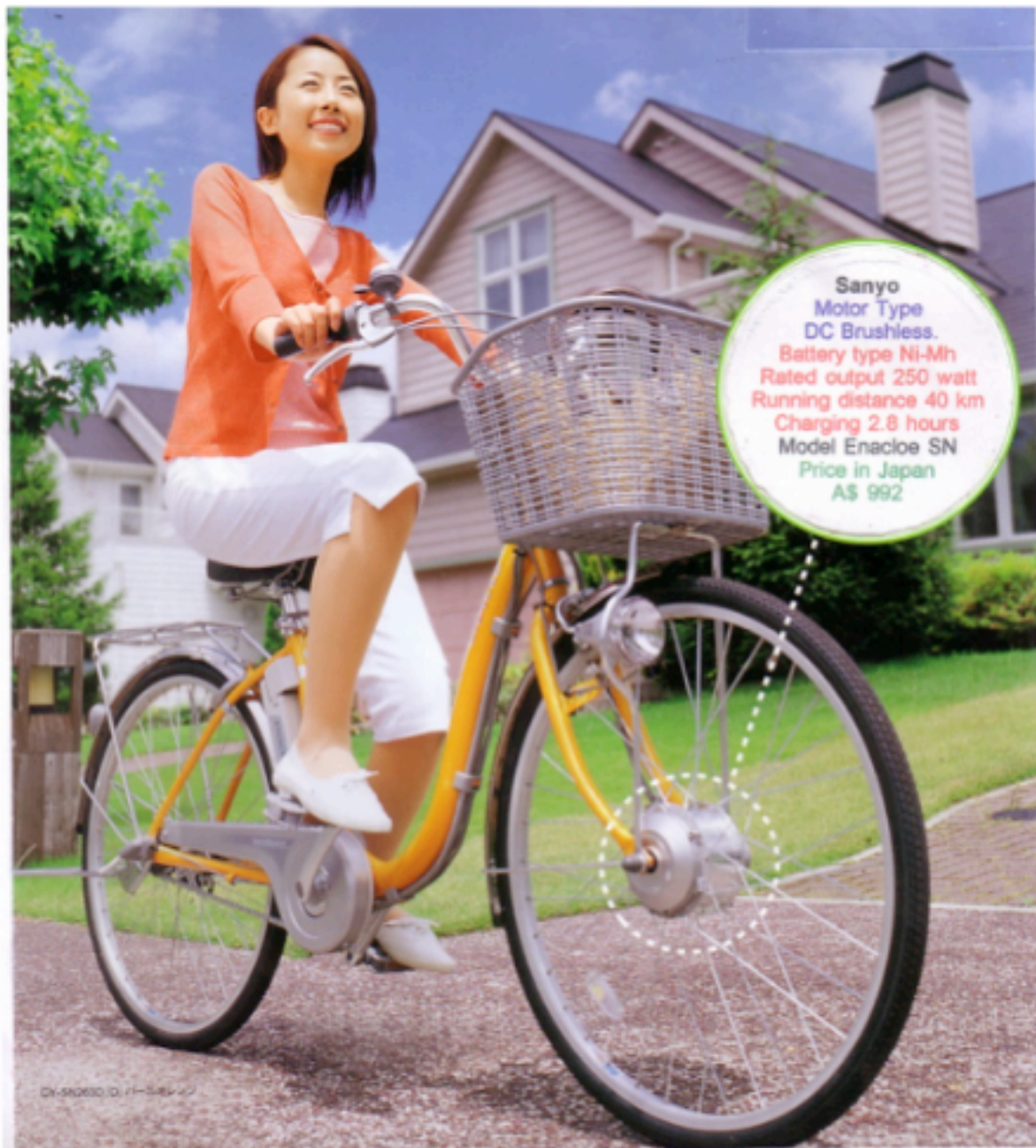
Figure 1 Sanyo electric PAB: 250 watt rated output Ni MH battery price today around a $1000. Note the small battery behind riders left foot.
